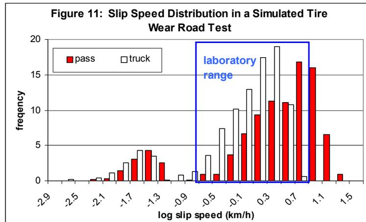
area i.e. on the forces on the tire and the slip stiffness of the tire. Figure 11 show slip speed distributions for a passenger car tire- and a truck tire road test respectively. It is obvious that the slip speeds are much lower than the driving speeds. They are naturally somewhat higher for passenger tire road tests than for truck tire ones but do not differ very much from slip speeds in the laboratory abrasion test which range from about 0.2 km/h to about 10 km/h.
