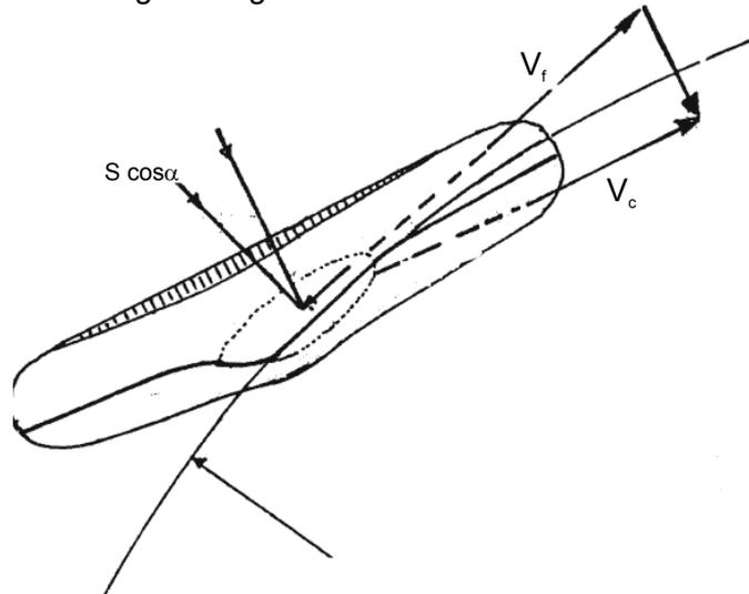
During steering the vehicle around a corner, the plane of the wheel makes an angle  $\alpha$  with the tangent of the cornering curve and side slip  $s$  occurs which becomes
