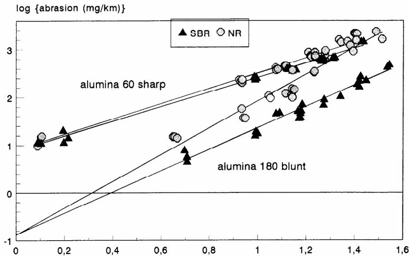
depend on the rubber compound and the sharpness of the abrasive track. This can result in cross-over between the ranking of compounds.
