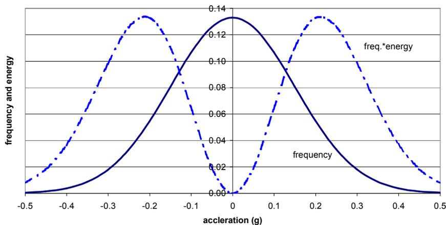
Also shown is the consumed energy multiplied by the frequency of its occurrence for a given tire stiffness and load (normalized to fit the scale). This is zero at straight driving, because there is no side force and it becomes zero again at very large accelerations because of their low or near zero occurrence.
