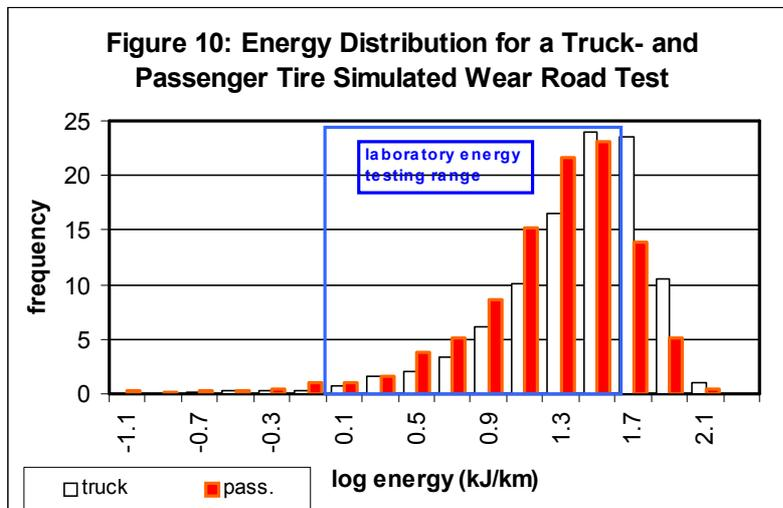
distribution of energy consumption in the contact area. Figure 10 shows such an energy
