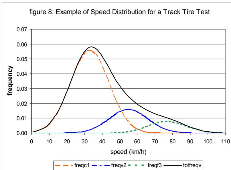
An example is shown in figure 8 for a truck tire test. The distribution is an example. Its exact shape depends on the prescribed testing conditions of maximum speed and the ratios of town, country and motorway driving. Figure 9 is an actually measured distribution. The shown simulation was obtained by two superimposed normal distributions i.e. the height of the third was taken to be zero.
