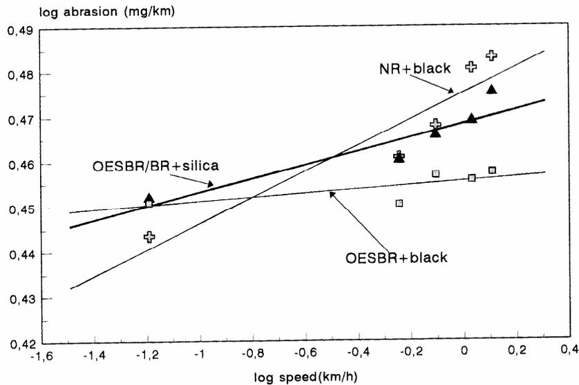
load). These lines, too, show cross over effects, indicating that compounds can reverse their ranking with speed at a constant energy dissipation as shown in figure 4 for three tread compounds based on different rubbers and fillers.
