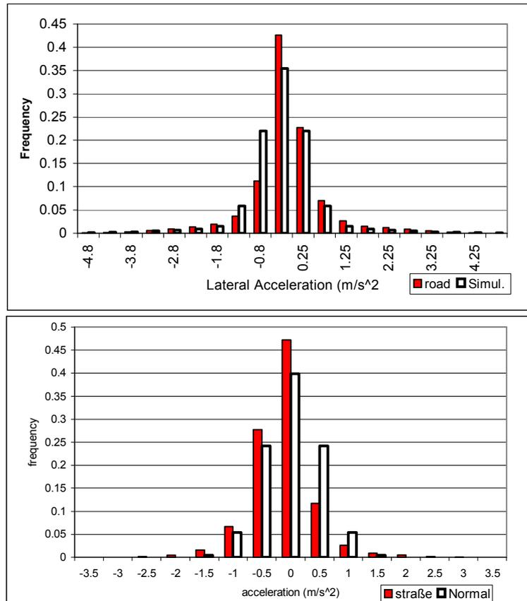
normally distributed around zero. They are defined by their standard deviation  $\sigma$ . If it is also assumed that the occurrence of the maximum acceleration during driving is  $3\sigma$  (99.9% of all occurrences), a measure is found for the driving severity due to applied forces. That such an assumption is close to reality is shown in figure 6, which compares actual acceleration measurements during a road test with a normal distribution function for lateral and longitudinal accelerations.
